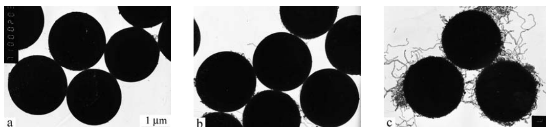
Fig. 2 TEM images of MWCNTs-coated PS composite particles prepared by different weight ratios of MWCNTs/PS, 1:25 (a), 1:10 (b) and 1:2 (c) (The scale bar corresponds to all TEM images)
